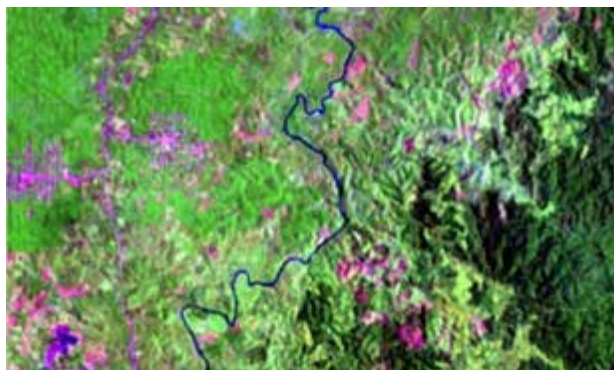
Figure 6. Landsat 8, results of stacking one year images from March 2017 to beginning April 2018, cloud and shadow were removed and the median value calculated for each pixel. This image represents a 2017 image.
