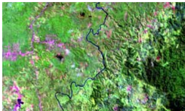
Figure 7. Landsat 8, results of stacking one year images from March 2018 to beginning April 2019, cloud removed and the median value calculated for each pixel. This image represents a 2018 image.
